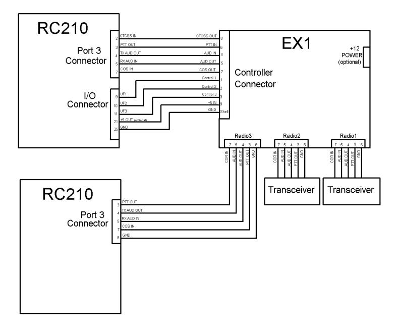
Port 3 of each RC210 should have both its COS and CTCSS Polarity Jumpers set to Active Low (Pins 1 & 2). Likewise, the EX1 should have its Port 3 COS Polarity Jumper also set to Active Low (ON).
