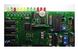
If you have the optional AP1 Intelligent Autopatch, plug its 8 pin connector into the RTC's JP2 connector, taking care to line up pin 1. That's it! Now power up your RC210 and set the clock and calendar (which should be the last time you ever have to do that!)
